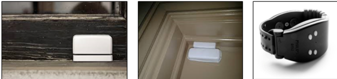
Figure 3-1: Images of the sensor types used for exercise detection. From left to right: SmartSense multi-sensor, Aeon labs door contact sensor, and DTI-2 wristband.
