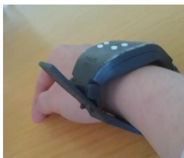
Figure 8: DTI-2 sensor was difficult to fit to smaller wrists
