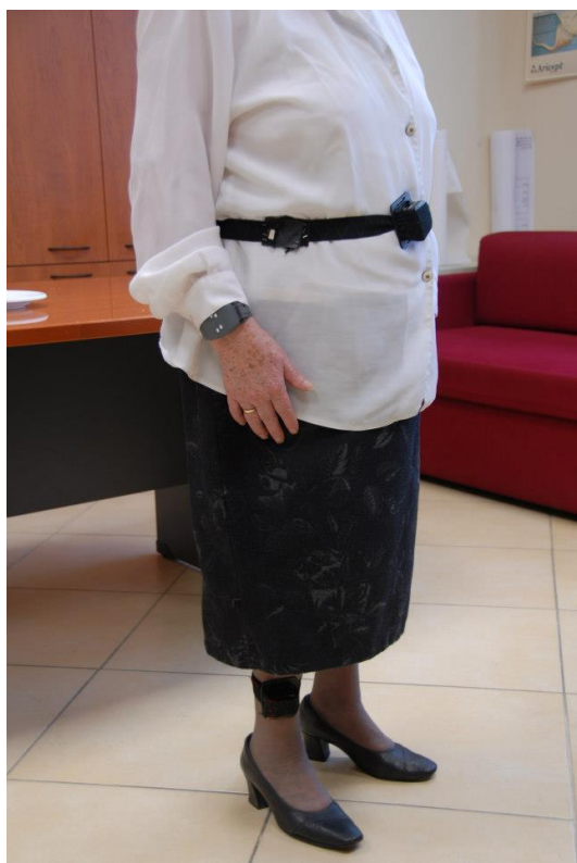
Figure 17 Left: Participant wearing WIMU sensors around her waist on her leg with DTI-2 sensor on her wrist (Source, Dem@care, 2013); Right Philips DTI-2 sensor
