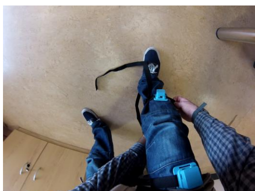
Figure 9. Screenshot from GoPro Camera illustrating the straps used to affix the WIMU sensors to leg and torso.
