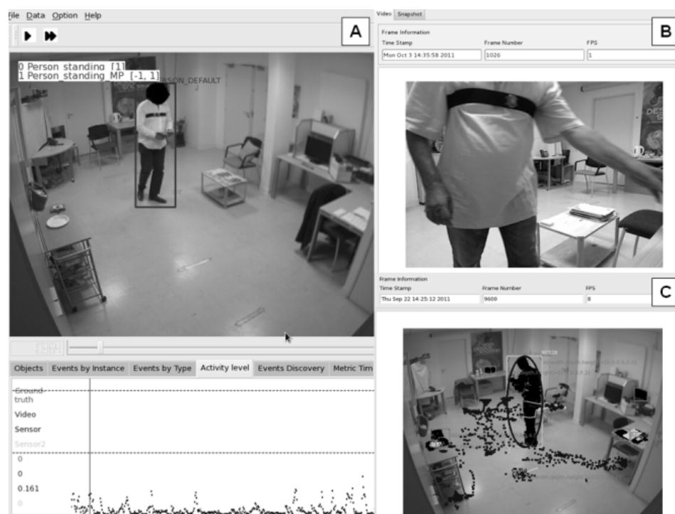
Figure 5-5 Recording viewpoints and example information: ambient camera view (A); RGB-D camera view (B), showing also in close-up the inertial sensor worn by the participant; actimetry information (bottom of A); trajectory information (C).
